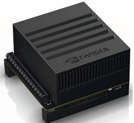
8. NVIDIA's Jetson Xavier can deliver 32 TOPS of performance for machine-learning chores.
